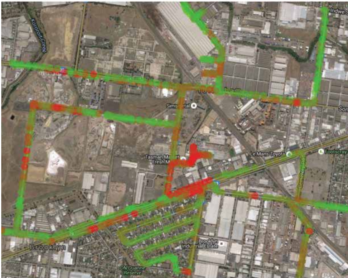
Mobile particle monitoring in Brooklyn. Green indicates low readings and red indicates high readings of dust particles.
